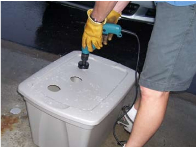
Cut holes in top of bin. You can use a drill, knife, or saw to do this. 4-6 holes about 2" in diameter will work for an 18-gallon bin. Smooth holes with sandpaper.
