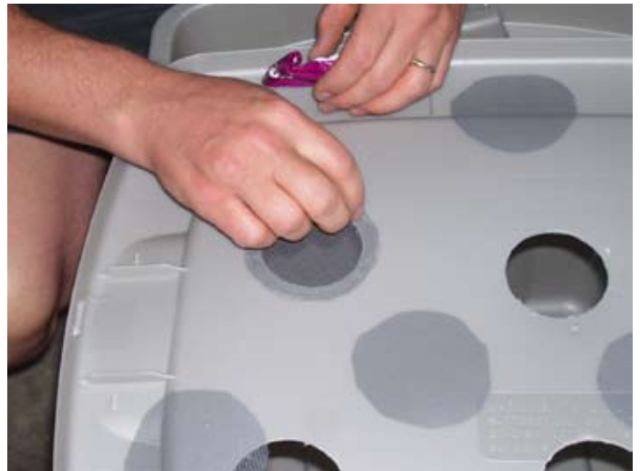
Cut screening material (screen, cheesecloth, pantyhose) to cover holes and secure with glue or tape.
